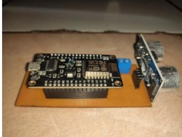
Figure 7. The IoT Node Use HC-SR04
