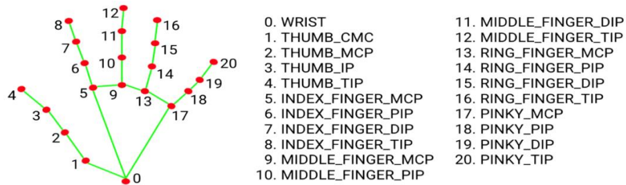
Figure 2. MediaPipe Hand Landmark Detection
